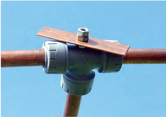
Fig. 4: The tuning vane is a brass or copper plate 80x20mm.
